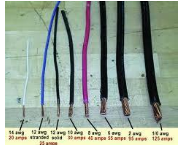
Wires come in different sizes. The maximum current each size can conduct safely is shown.
