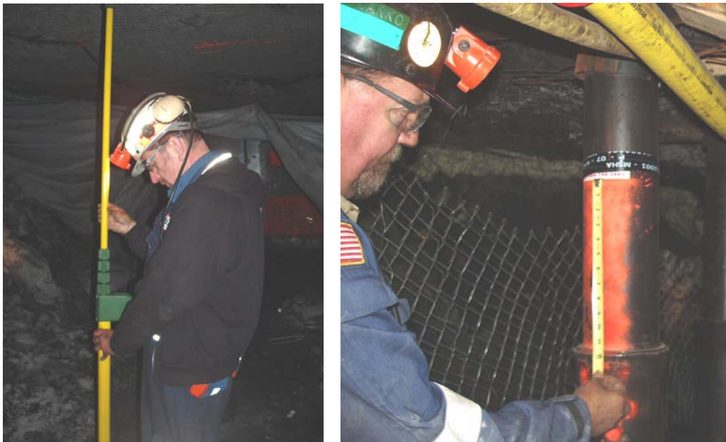
Figure 95 - Convergence Measurements Left: Roof-to-floor convergence station. Right: RocProp convergence station.
