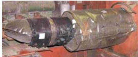
MineWrap™ Covering Exhaust and Catalyst
