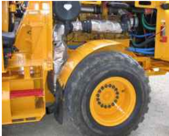
Mining Vehicle, Exhaust & Catalyst Insulated
