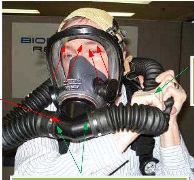
Tests integrity of exhalation check valve!
