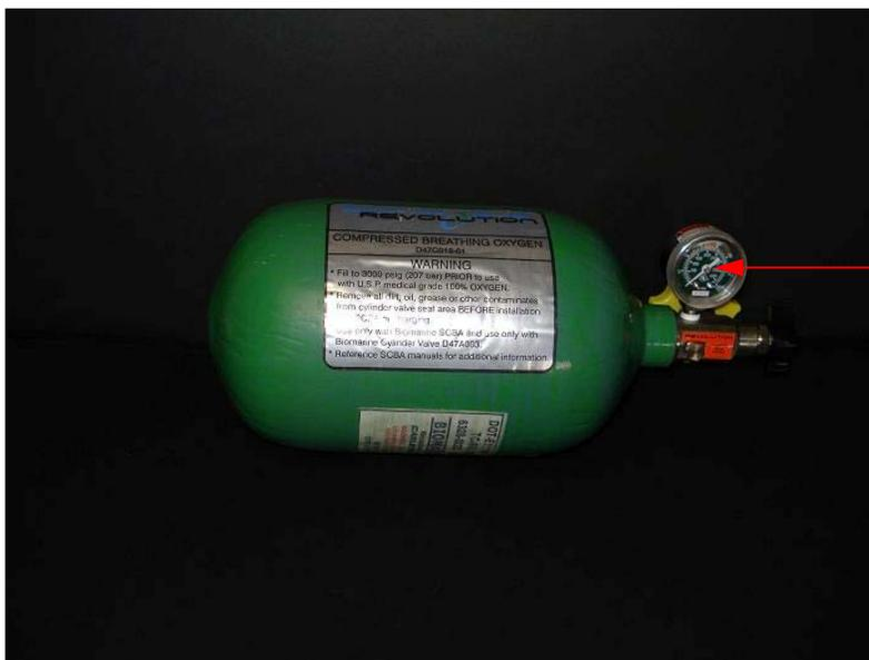
3000 psi minimum for a 4-hour capable CCBA.
