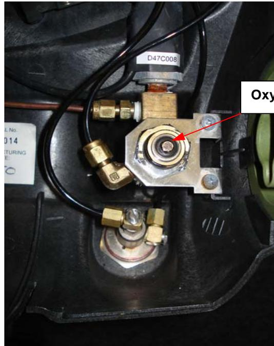
Oxygen cylinder washer seal
