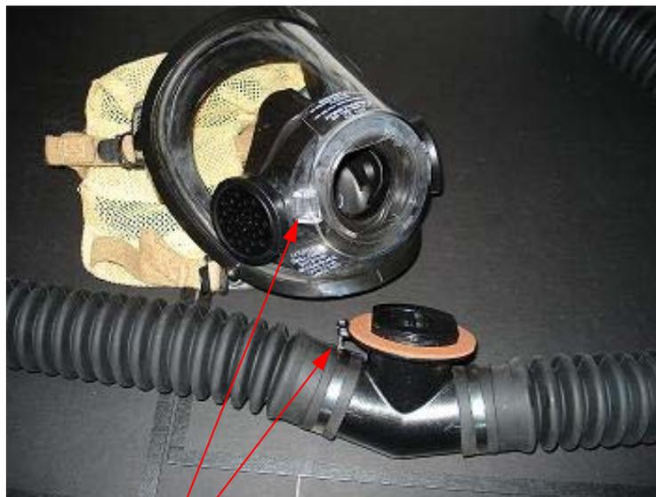
Once the adapter is installed on the face piece, engage the slide lock into the mask slide lock channel.
