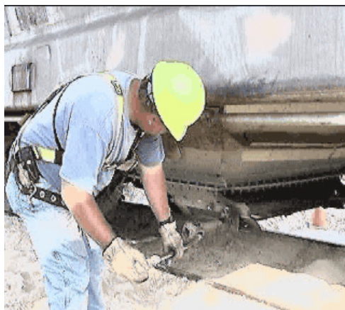
Figure 29.—Using steel bar to open hopper gates ( left ); gates opened via mechanical assist ( right ).
