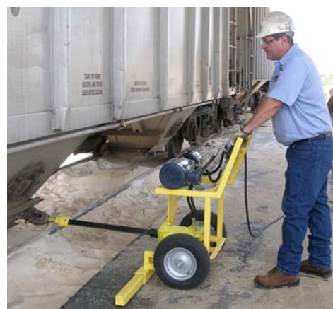
Figure 29.—Using steel bar to open hopper gates ( left ); gates opened via mechanical assist ( right ).
