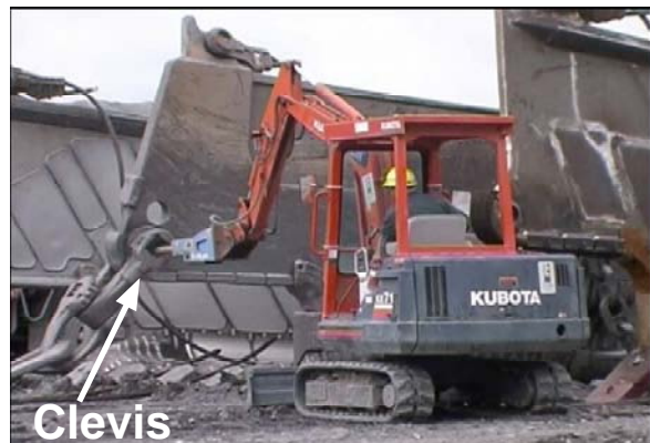
Figure 25.—Clevis pin removal: (A) manual removal with a sledgehammer; (B) removal using machine-mounted jackhammer.
