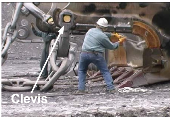
Figure 25.—Clevis pin removal: (A) manual removal with a sledgehammer; (B) removal using machine-mounted jackhammer.
