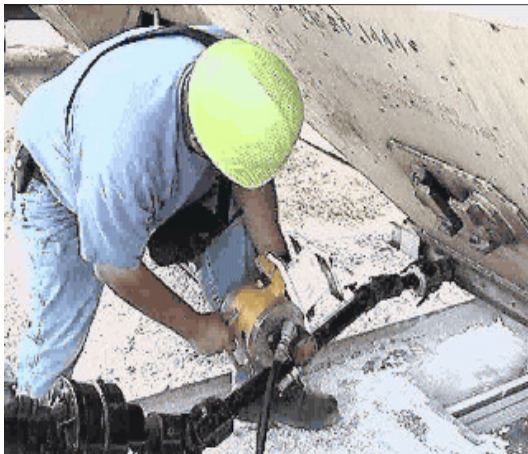
Figure 30.—Installing railcar shaker involves heavy load in flexed posture ( left ); a simple device can be used to install shaker with a minimum of effort ( right ).
