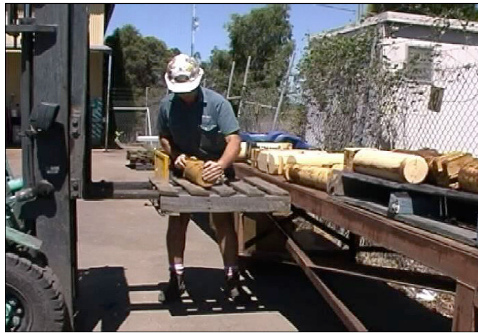
Figure 24.—Using forklift and pallet for easy transfer of loads.
