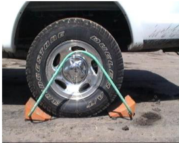
Figure 28.—Attaching a simple handle to wheel chocks greatly reduces excessive bending to place or remove the chocks [Torma-Krajewski et al. 2006].
