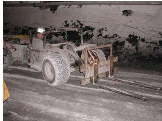
Figure 31.—Well-organized trays ( left ) can be efficiently transported underground using scoop-mounted forks ( right ).
