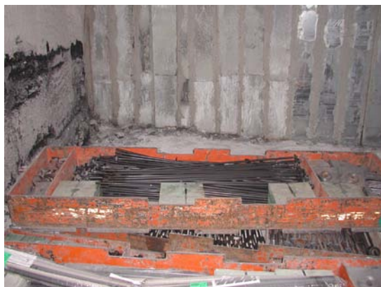
Figure 31.—Well-organized trays ( left ) can be efficiently transported underground using scoop-mounted forks ( right ).
