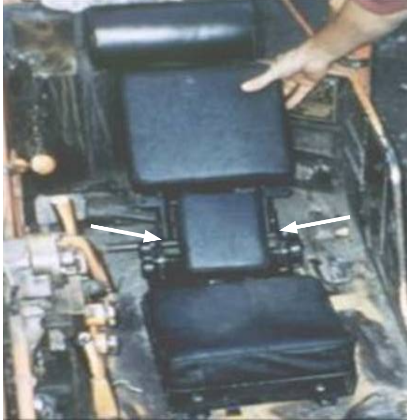
Figure 39.—Prototype seat design for underground mining equipment. Note cutouts in the seat backs (indicated by arrows) to accommodate belt-worn PPE [Mayton et al. 2006].
