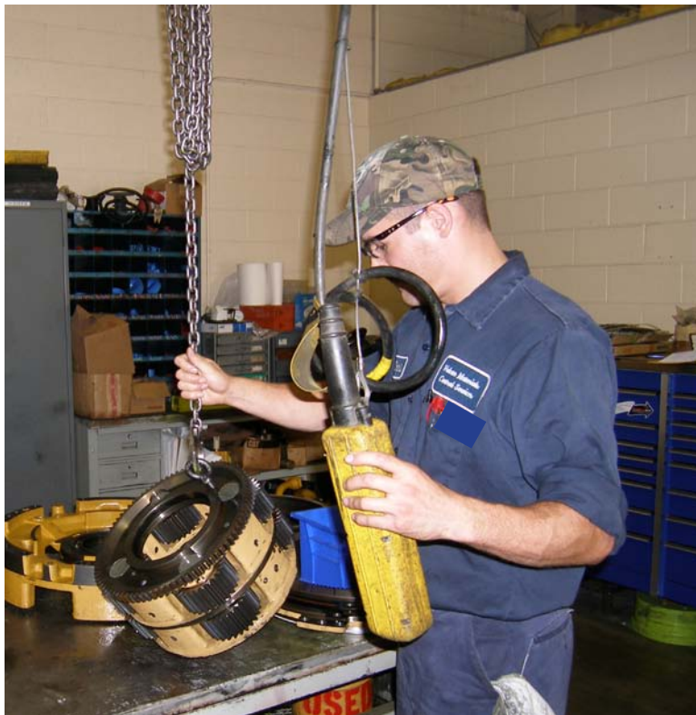
Figure 21.—Hoists can be used at many locations on the surface and underground to lift heavy items.
