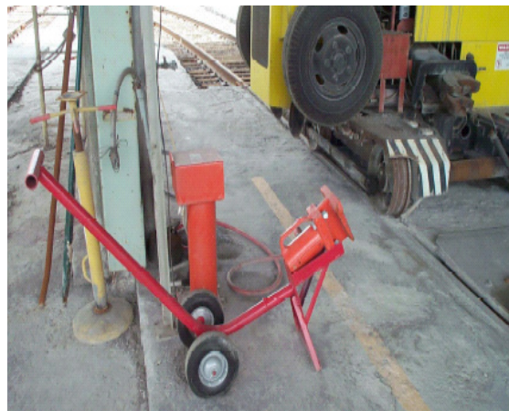
Figure 30.—Installing railcar shaker involves heavy load in flexed posture ( left ); a simple device can be used to install shaker with a minimum of effort ( right ).
