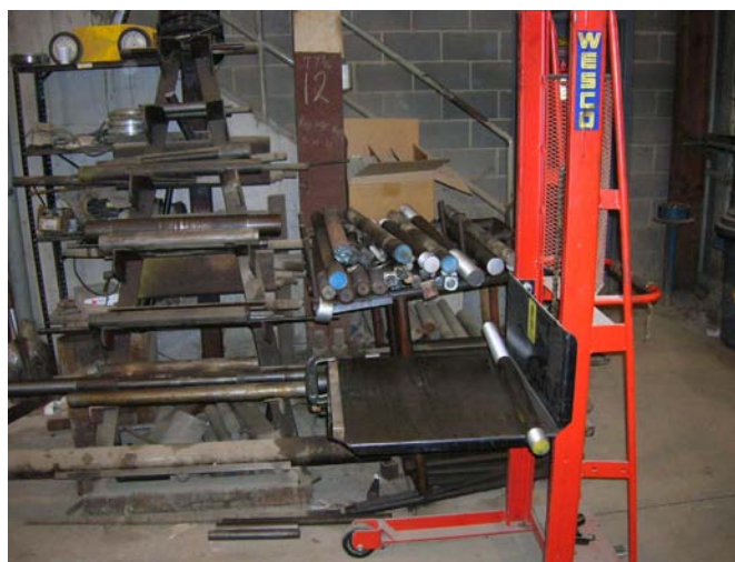
Figure 27.—Lift stands can have many uses in shop areas and can greatly facilitate load transfer.
