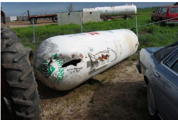
Tank ruptured and left its running gear
