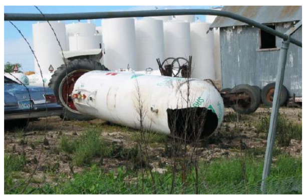
Tank split a tractor in half before coming to rest
