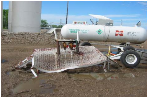
Tank ruptured and left its running gear
