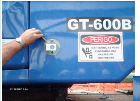
The automatic safety interlocks for the crane operation were immobilised at the key outside of the operators cab by the crane operator.
