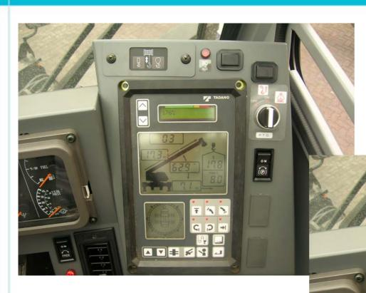
The crane operator had a history of overriding the crane limits and overloading the crane. Shown by computer records from the crane over 40 overloading incidents during October 2007
