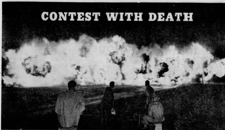
Four hundred pounds of coal dust goes up with a roar in a simulated mine explosion at state fairgrounds. Blast opened event.
