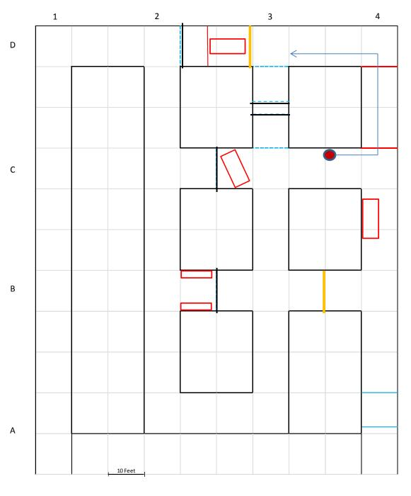
In order to explore behind the barricades for the two missing miners the team will need to ventilate the mine. Ventilation is as simple as sealing the fire, building one stopping and turning on the main, then the auxiliary fan.
